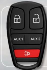
The MV™ Series features a programmable key fob that allows two Diamond Logic tasks (such as pre-trip light inspection) to be activated with the push of a button
