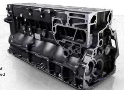
The crankcase is constructed with North America's first big bore Compacted Graphite Iron (CGI) design for 75% higher tensile strength and 45% greater stiffness while reducing weight, noise and vibration.
