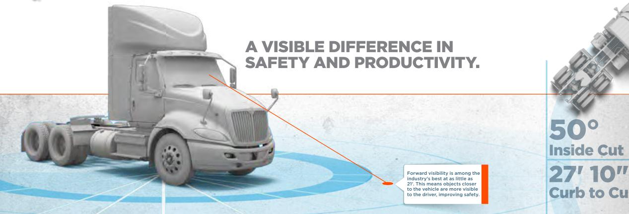
The RH Series interior was designed based on a meticulous study of interaction points between the driver and truck - everything from what a driver sees to how he moves and reacts in virtually any situation. That's why the RH Series has been designed with a large swept-back windshield, optimized mirror placement and an aerodynamic sloped hood for a clearer view.
